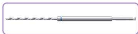
Drill Bit, \varnothing 2.0 \times 125 mm, Stop 50 mm, Stryker Coupling, Barrel \varnothing 4.5 mm, Blue Code
